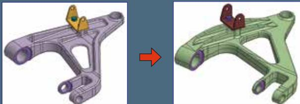
CATIA V5 has tools to enable easy replacement of components in an assembly. When using publications, the Abaqus analysis model automatically updates with the new geometry.
